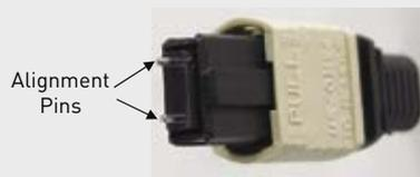
The pinned connector is typically located inside the panel to help protect the pins from being damaged (i.e. the fixed connector is pinned and the connector that is frequently removed and handled is unpinned). For example, cassettes are typically pinned and trunk cables are typically unpinned.
