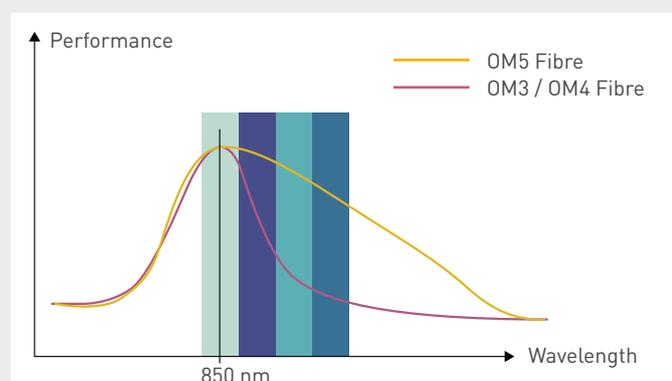
As was mentioned, Phase I of the 400GbE (IEEE 802.3bs) standard will specify transmission over multimode using parallel transmission with a channel rate of 25 Gbps. This will require a total of 32 fibres. Employing SWDM over WBMMF reduces the fibre count to 8 fibres, 25% of the number of fibres required in Phase I.
