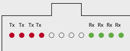
The 100GBASE-SR10 (100 GbE over multimode) requires a total of 20 fibres, 10 transmit and 10 receive. Position assignments are shown below. There are three options, the first being a single receptacle shown as Option A in figure below. Option A is recommended by IEEE. The two-receptacle options: Option B and Option C are alternatives.
