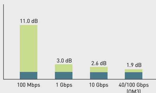
■ Margin between the link loss and the application limit
