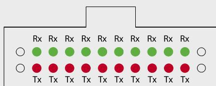
Option B and C use two 12-position MPO connectors. Option B, shown in the figure below, uses side-by-side interfaces. The 10 middle positions of the right-hand interface are used for reception and the 10 middle positions of the left-hand interface are used for transmission.
