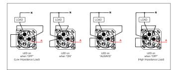
Note: Low Impedance Load examples include incandescent, halogen, resistive loads. High Impedance Load examples include CFL's, LED globes.
