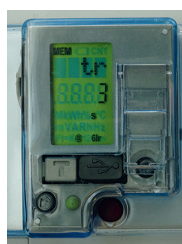
Time delay on current setting.
