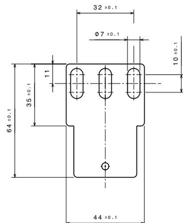
Fixing centres (min.-max.) with standard brackets : 1554mm -1574mm
