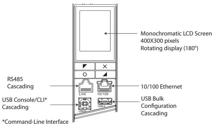
Node controller is plugged on the base and is hot swappable.
