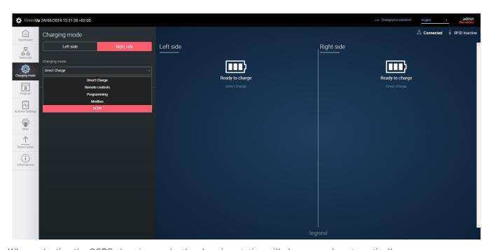
When selecting the OCPP charging mode, the charging station will change mode automatically.
