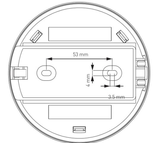
Fig.4: Mounting hole pattern on base
