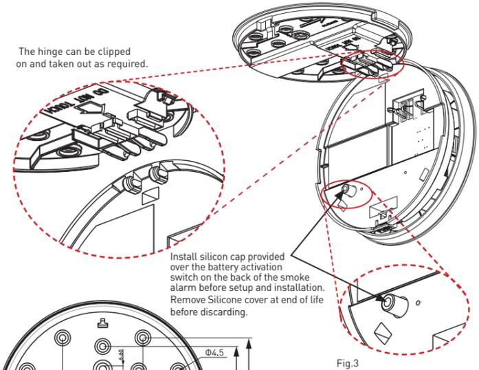
The hinge can be clipped on and taken out as required.
