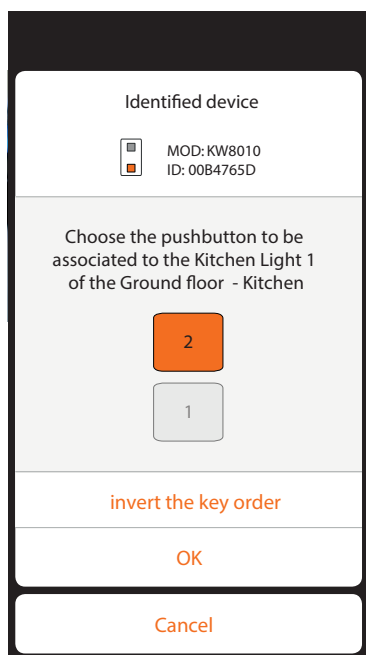
Activation of the MyHOME_Up system - definition of the LIGHT command for the control of two lights.
