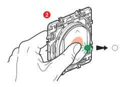
**Briefly** press the wireless control to activate it. The indicator light will flash green and then switch off.
