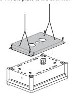
5. Fit the power cable through the gland and terminate into the terminal block.
