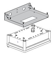
4. Fit the power cable 1 through the gland and terminate into the terminal block.
