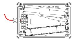
5. Fix the box to the ceiling through the 4 lugs. Use 10 to 14 gauge screws (not supplied).
