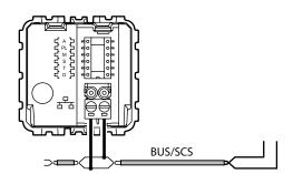
Pressing the auxiliary control enables the load to be switched on or off manually. If the control is not pressed, the sensor will cut off the load at the end of the time delay or when the light level threshold has been reached.
