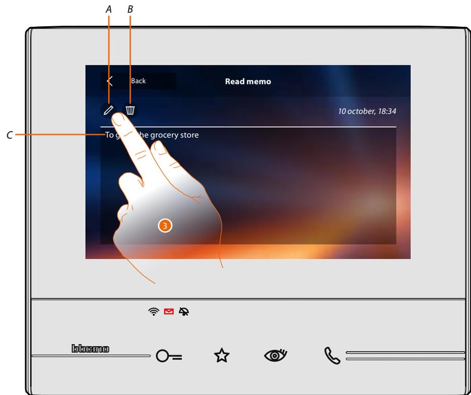
This screen can be used to display (C), modify (A) or delete (B) the memo text.
