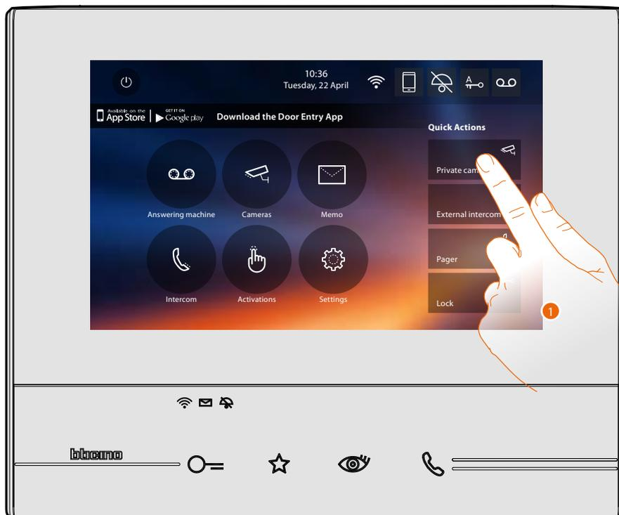
1. Touch to directly enable the function (e.g. camera).
