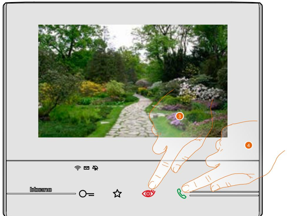
3. Touch to display another camera (scrolling). When switching from one camera to the next, the key lights up.
