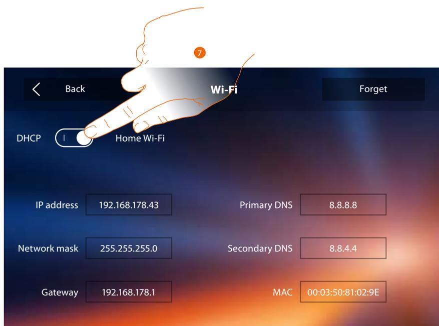
7. Touch to disable the DHCP mode and to manually modify the parameters.
