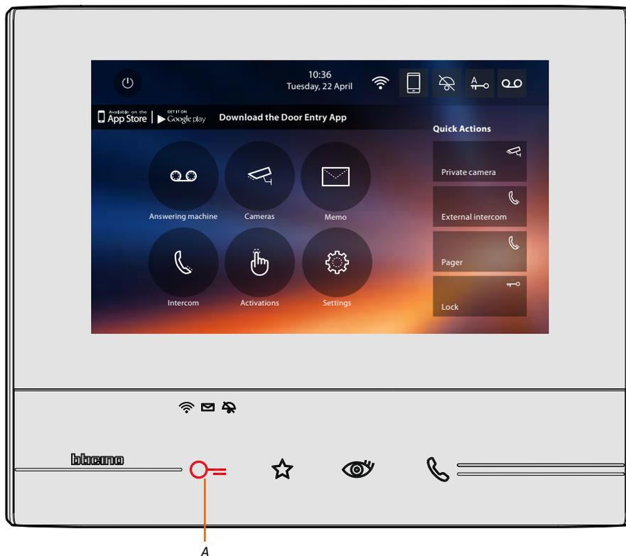
A. LED flashing = door lock open.
