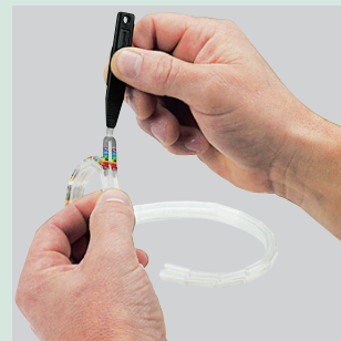
3. Installation in double marker-holder
