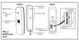
the first 6 switches located inside the Bell Press Battery Compartment (Fig. 2 K). Remove the Bell Press [Fig. 2 G] from the Mounting Bracket (Fig. 2 J). Open the Battery Compartment cover on the back of the Bell Press. Select a different channel by moving one or more of the 6 Channel Selection Switches to the ON position.
