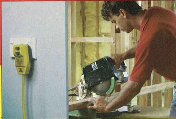
Cutting tools are capable of cutting their own electrical leads. Provide the tool with permanent protection.
