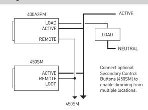
**Note:** An unlimited number of 450SM can be connected to an 400A2PM. However, the total length of the remote wire used to interconnect all of the 450SM should not exceed 50 metres.
