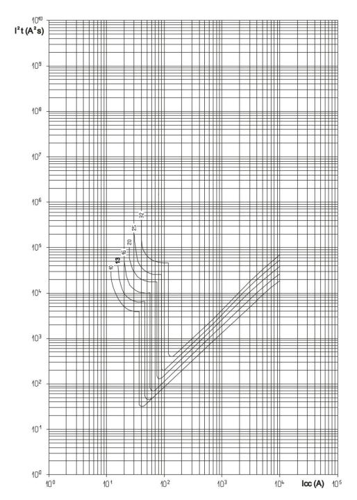
lcc = Prospective short-circuit symmetrical current (rms value in kA)  $I^2t$  = Limited thermal stress (in A²s)
