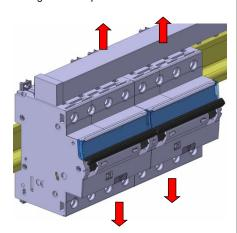
Put the clamp in the unlocking position
