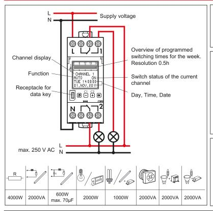
Operating principle: Typ 1.B. S. T. IEC/EN 60730-1, IEC/EN 60730-2-7 Operation in a normal environment
