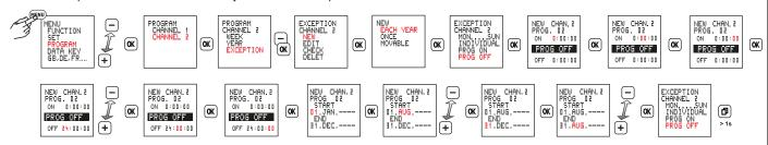
2 Each year from 25.12. to 26.12., the output is to be switched on at 6:00 hours, switched off at sunrise, switched on at sunset and switched off at 23:00 hours. For this, two programs are needed:
