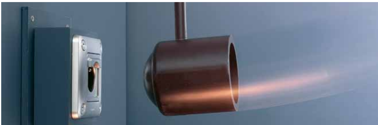
IK 10: MAXIMUM IMPACT RESISTANCE | All Soliroc products can withstand impacts of 20 joules
