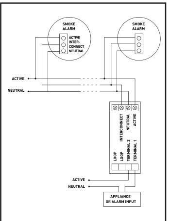
Figure 1. Wiring diagram for 643086.
