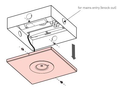
Step 3. Install the unit onto the ceiling using the mounting holes shown below.
