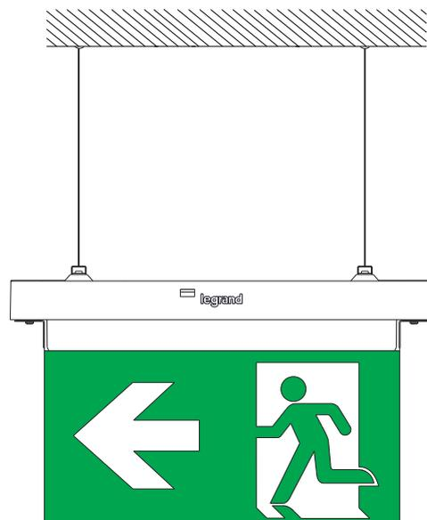
Fix the screws from inside (screws provided with the kit)
