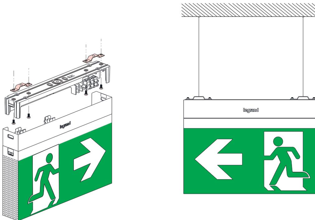
Fix the screws from inside (screws provided with the kit)
