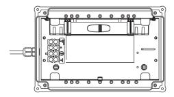
**Note:** For wireless models, the antenna should be facing away from the gear tray. For DALI models, connect the two DALI wires to the DALI terminals.
