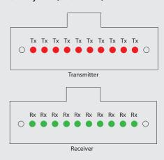
Options C is similar to option B, but uses the stacked layout depicted in the figure below. The ten middle positions of the top connector are used for reception and ten middle positions of the bottom connector are used for transmission.
