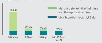
It is important to consider the trade-off. If the IL of one component can be reduced, there will be room for extra loss in another component. For example, if using OM4 at only 100 m instead of 150 m. the loss of the cable will be less because IL is directly related to distance (dB/km). This can make room for more mated connector pairs. However, all of the IL gain can easily be negated with inferior connector components.
