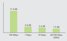
If we look at two channel insertion loss budget examples for 2 and 3 mated pairs, including the cable loss for a 100 m link at 850 nm, the importance of connector loss is apparent.
