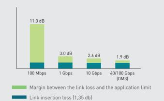
If we look at a 3-connector-pair channel, the loss budget rises to 1.85 dB ((3.5 db/km \* 0.1 km) + (0.5 \* 3)), as shown in the figure below. This is more than 70% of the 10 Gbps budget and almost the entire 40/100 Gbps budget. This would exceed the loss budget using OM4 for 150 m, which is 1.5 dB because of the longer distance, proving the insertion loss of a connector is very important.
