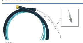
Supplied with pulling element. In coil up to 50 m, on a small drum between 51 m and 150 m, on a large drum over 151 m and up to 200 m Connection in fibre optic drawers and splice cassettes. OM3 aqua LSZH sheaths. Supplied with test reports
